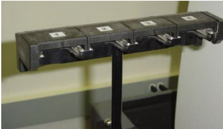
Renishaw SP 600 Stylus 更换架 ( SCR600 )
